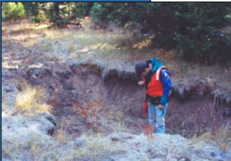
Rene Leclerc with Northwest Hydraulic Consultants, Inc. examining a knick point at the head of Clear Creek (photographer: Jeff Peters, Jones & Stokes).
